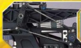
Elevator push-pull control system
