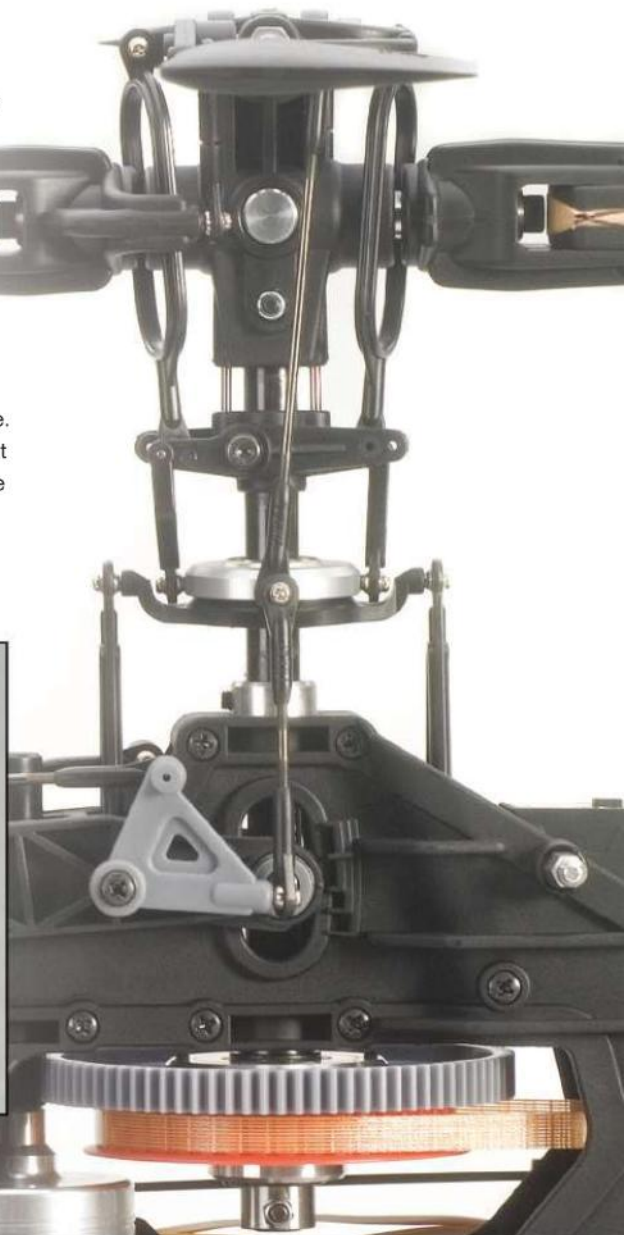
Greasing your thrust bearing is pivotal to prevent future failure.
